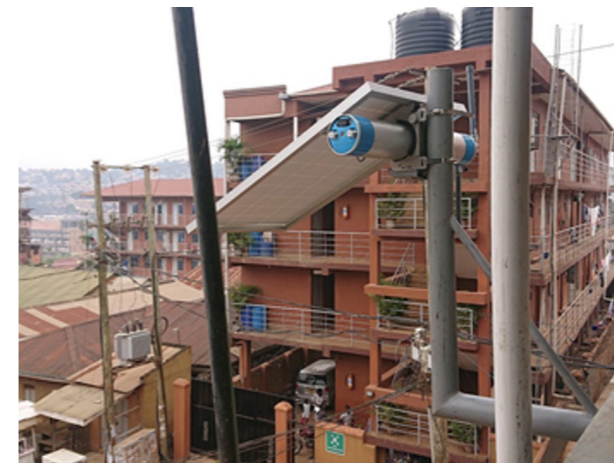
Fig. 10. Solar-powered router installed at a university hostel.
