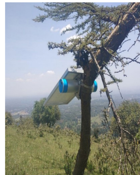
Fig. 11. Solar-powered router installed in the game park.
