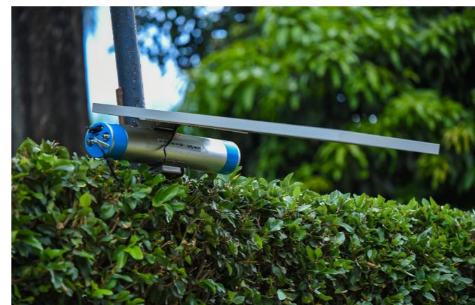
Fig. 9. Solar-powered router at Speke Resort Munyonyo.
